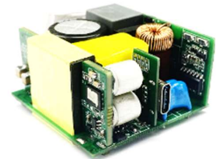
~750 kHz peak Half-Bridge GaN IC 120 W, 44 cc
