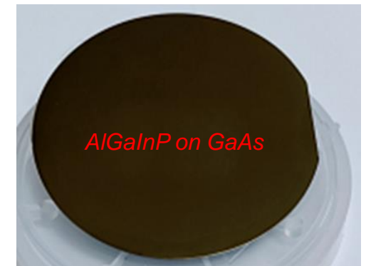
Epi wafer for red LED
