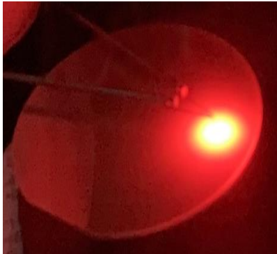
Red emission image of GaN-based epitaxial wafer grown on PSS (pattered Sapphire Substrate)
