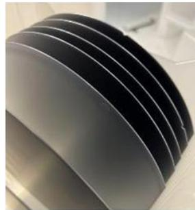
High-quality GaAs, InP, and GaSb templates grown on up to 12-inch Silicon substrates for scaling high-performance technologies to larger wafer sizes.
