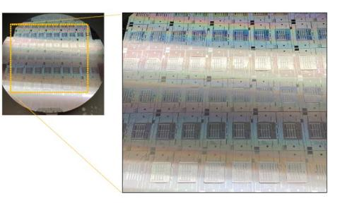
PhotonicBump – Imprint inside 20µm on 8" SiPh wafer
