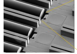
PhotonicPlug fiber connector
