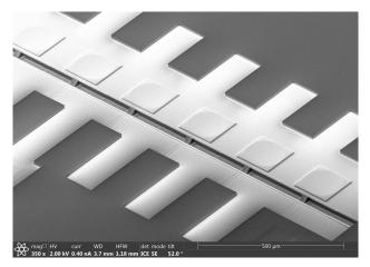
WLO for wide-band surface coupling, mode conversion and wafer level inspection.
