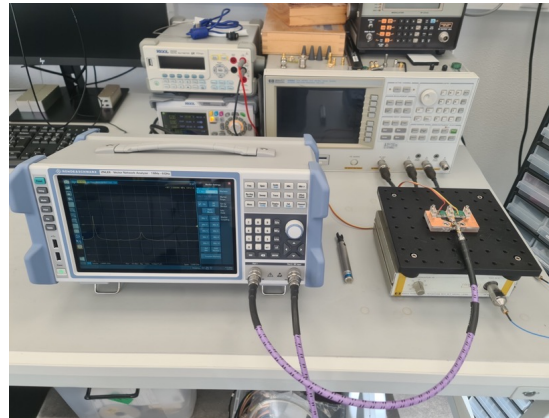
RF output impedance of modules being characterised in our lab.
