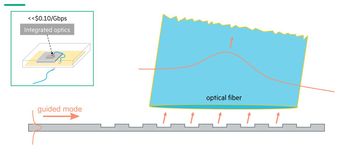
Typical Insertion Loss  $\approx -1.0$ dB (80% Efficiency)
