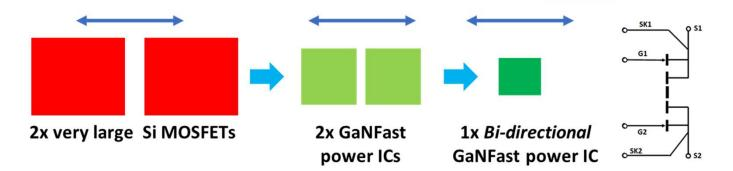
4x smaller than SiC Bidirectional FET, 3x smaller than two unidirectional GaN, 9x smaller than Silicon
