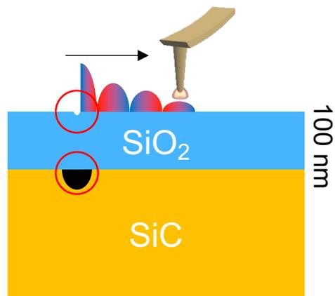
Surface phonon polaritons due to buried defects
