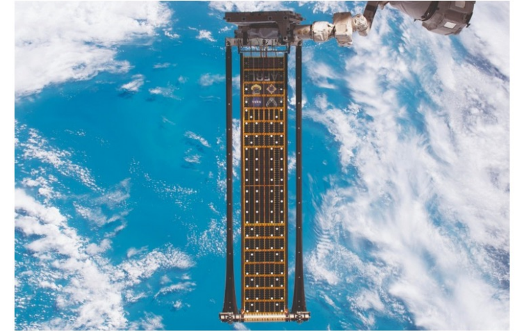
Flexible solar cells are needed on the ROSA (Roll Out Solar Array) held by the robotic arms at the International Space Station.
